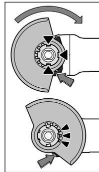
Place the protection guard **6** onto the spindle collar of the machine until the encoding keys of the protection guard agree with the spindle collar. Press and hold the release lever **1** while doing this.
